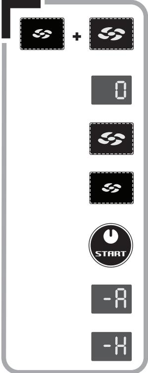
The diagram shows a vertical sequence of button presses: two cooling buttons (one with a plus sign), a display showing '0', a cooling on button, a cooling off button, a start button, a display showing '-A', and a display showing '-H'.
